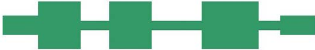
(c) Microstrip-line filter layout.
