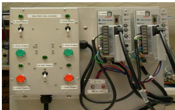
Fig. 1b Control panel and servo drives
